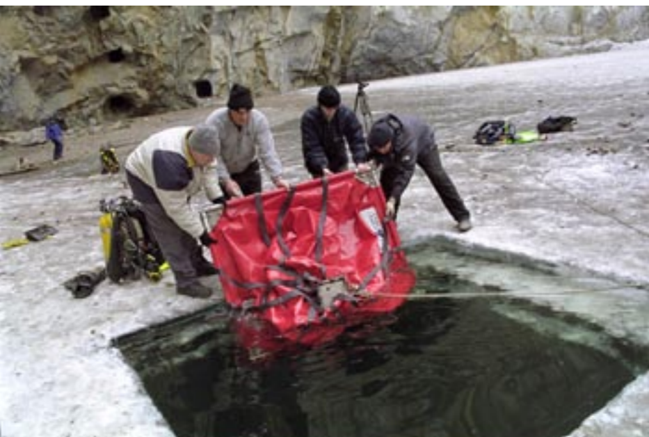
Divers place a soft underwater chamber under the ice
