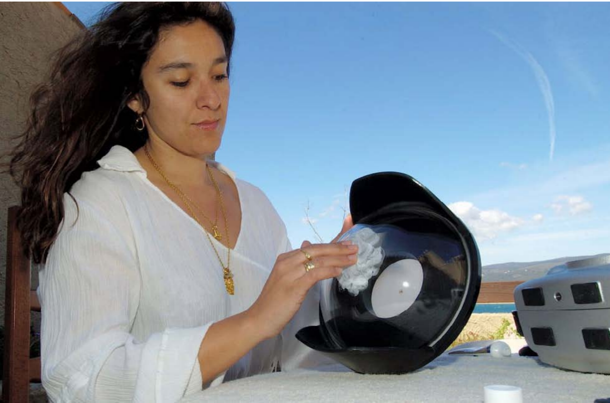
Ports/domes made of acrylic glass are easy to polish, but only on the outside. Never touch the inside, not even to polish
