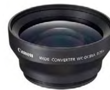
Canon Powershot wide converter (for a compact camera). Turns a 36mm lens into a 27mm by 0.75x magnification
