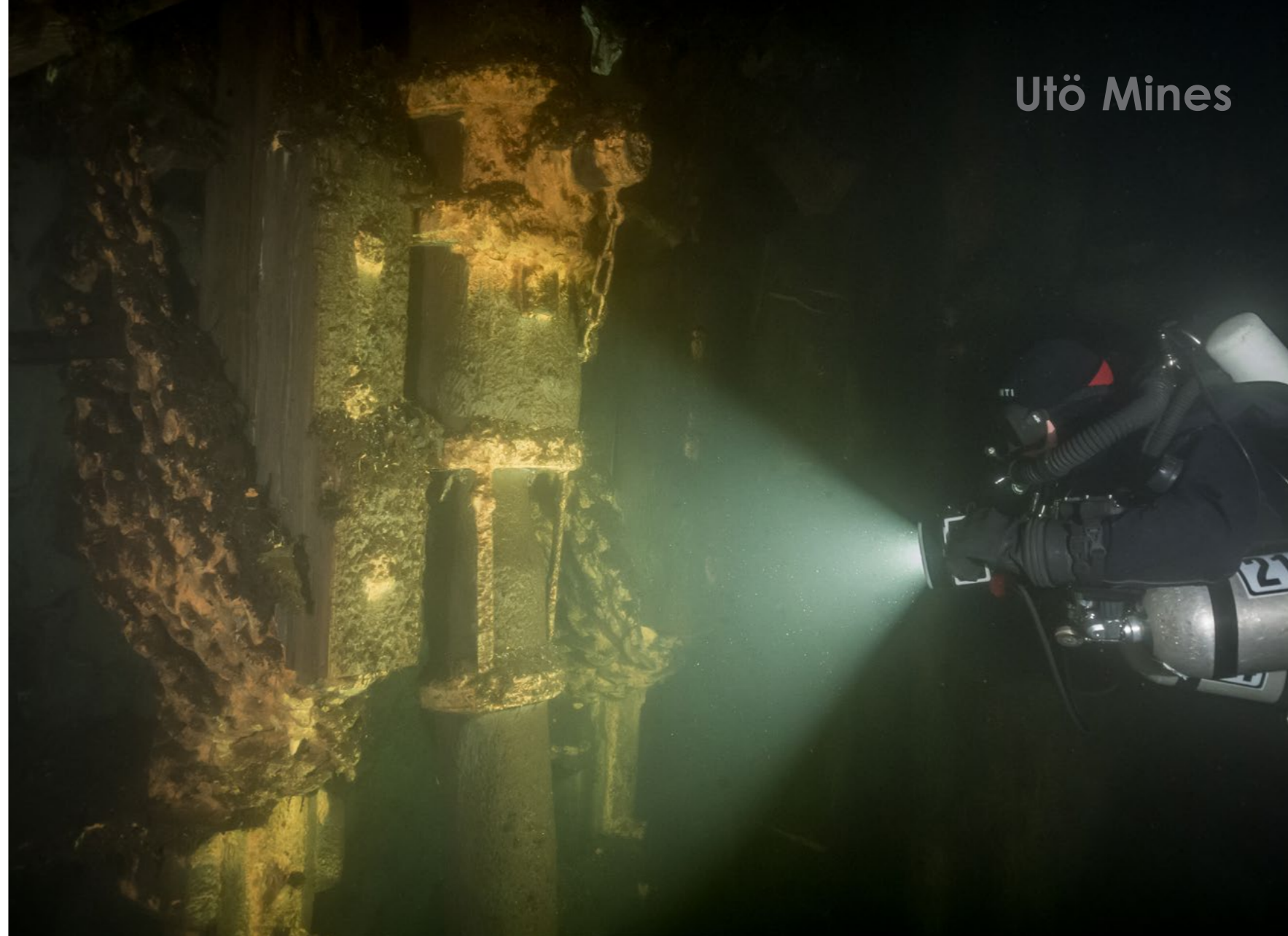
One of the cars, which were notorious on the island, was found at the bottom of Spensgruvan, 85m below the surface (above); The connection between two log pipes in the steam-powered pumping plant found in Finngruvan (Finn Mine) at around 60m (right)
