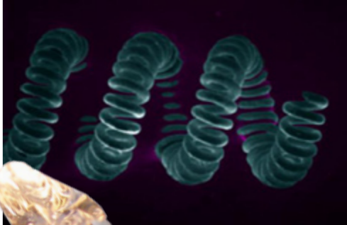
Scanning Electron micrograph of a light bulb filament (75x)
