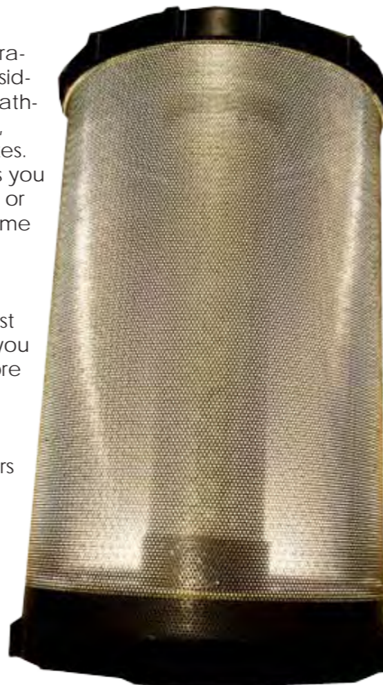
Golem Gear's radial scrubber unit for the Megalodon CCR is almost a piece of art. The breathing gas comes down the center axis and then traverses radially through the absorbent and through the grid
