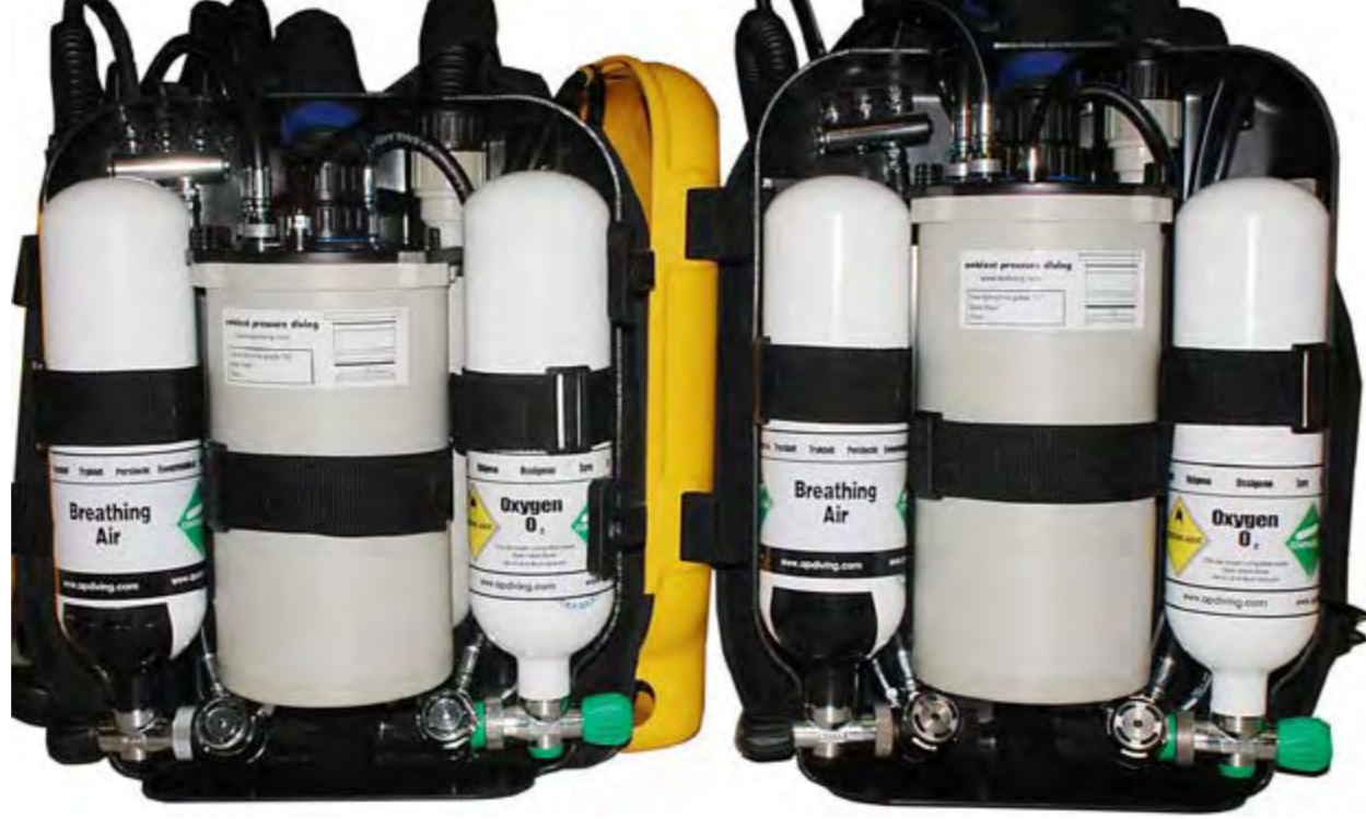
This photo is meant to illustrate the differences in length between the Evolution and Evolution+ scrubbers but also clearly shows the typical tank configuration. The oxygen tank is on the right. The diluent—in this case, air—is on the left. Tanks shown are 2-liter
