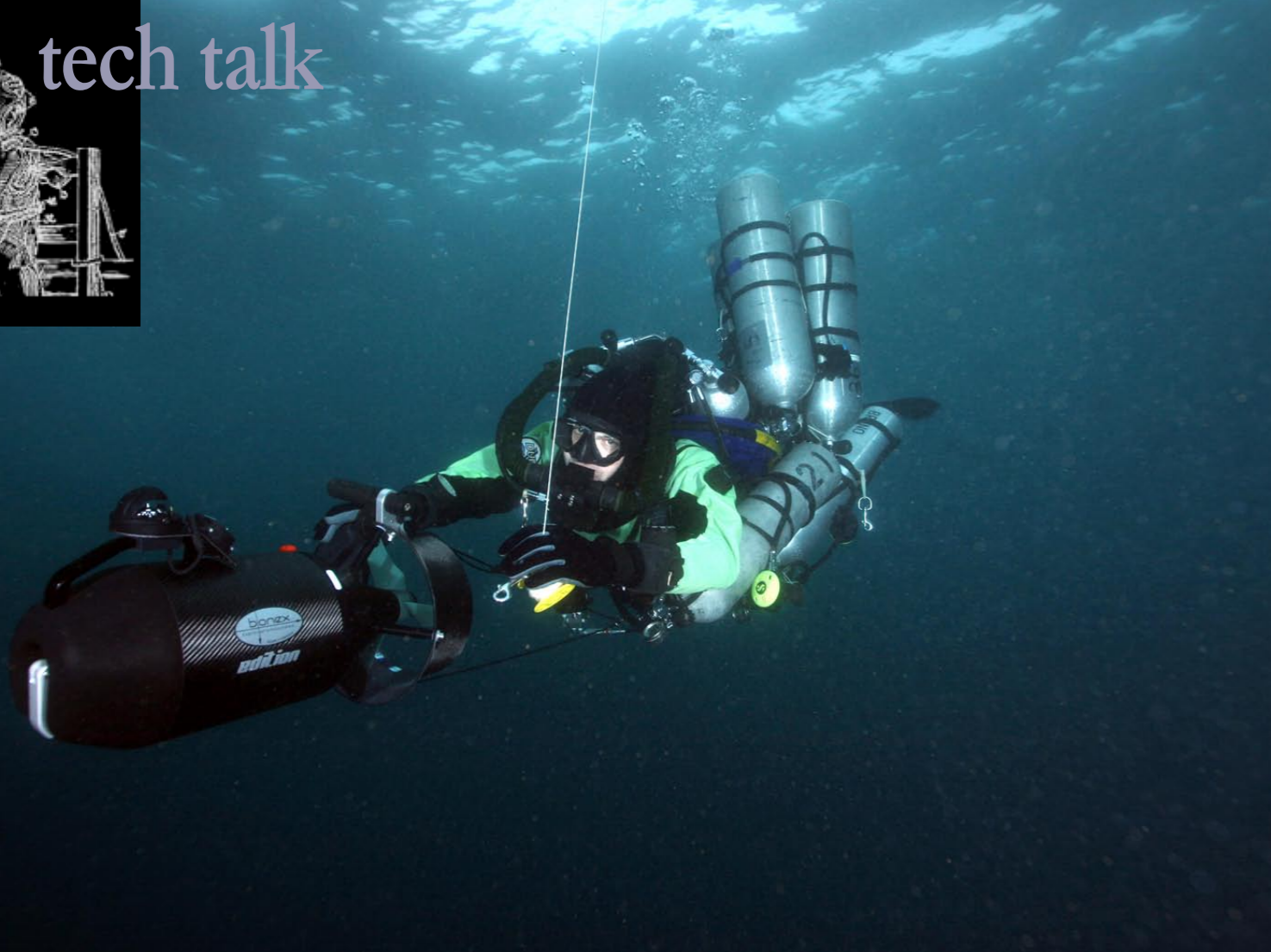
Technical diver on Semi-Closed Rebreather (SCR) with four stages and underwater scooter
