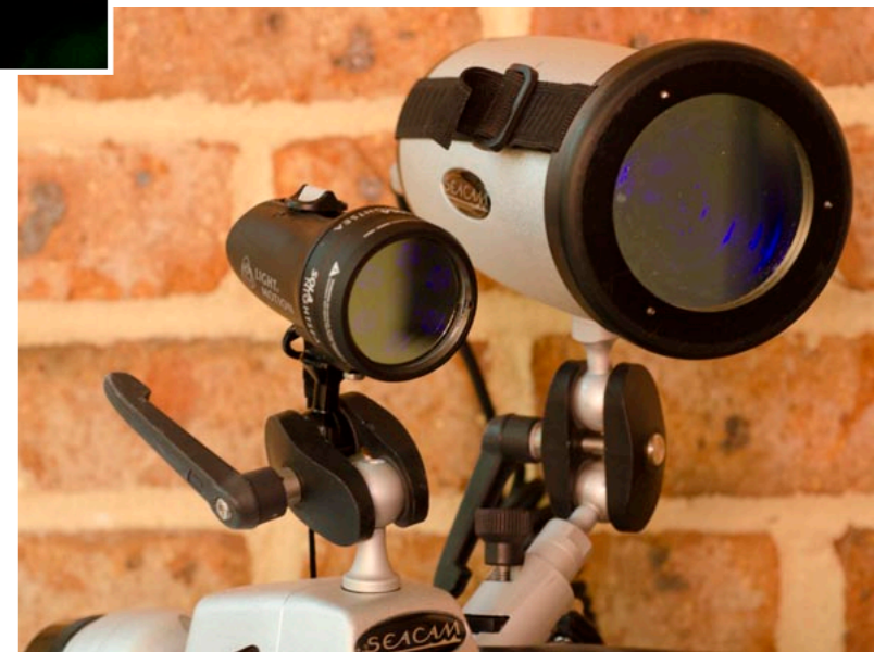
Fluorescing tropical coral polyps (left); The Sola Nightsea Light (right) provides a dedicated fluoro light wavelength. The Seacam strobe is fitted with a general purpose Nightsea Fluoro Excitation filter. These are available in a range of sizes to suit many strobes including Ikelite DS160/161
